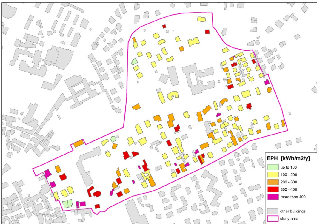
Figure 8. Heating energy demand computed with data package DP2. Image source: authors.
