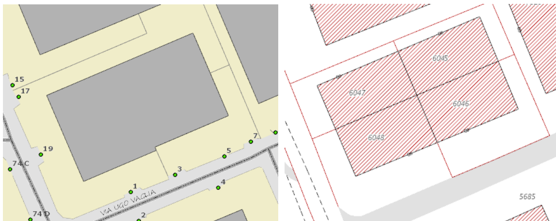
Figure 1. Example of a single building in the Topographic Database (TDB) (on the left), subdivided in four properties in the cadastre (on the right). Image source: authors.
